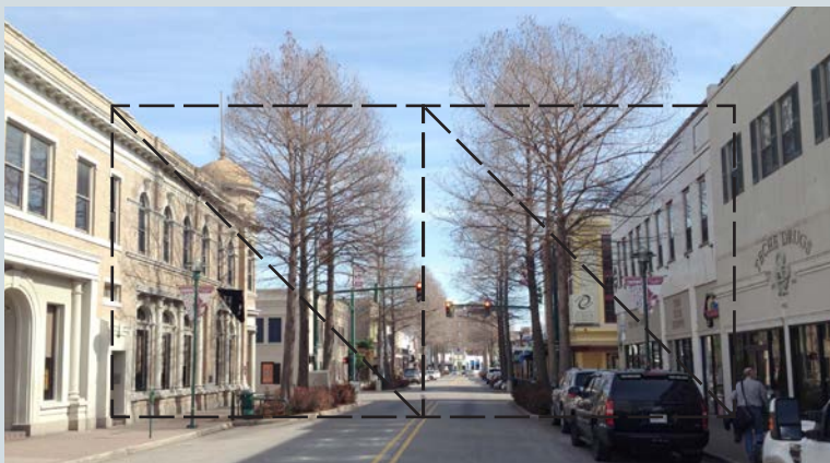
Jefferson Street achieves a 1:2 Ratio (Height:Width)
