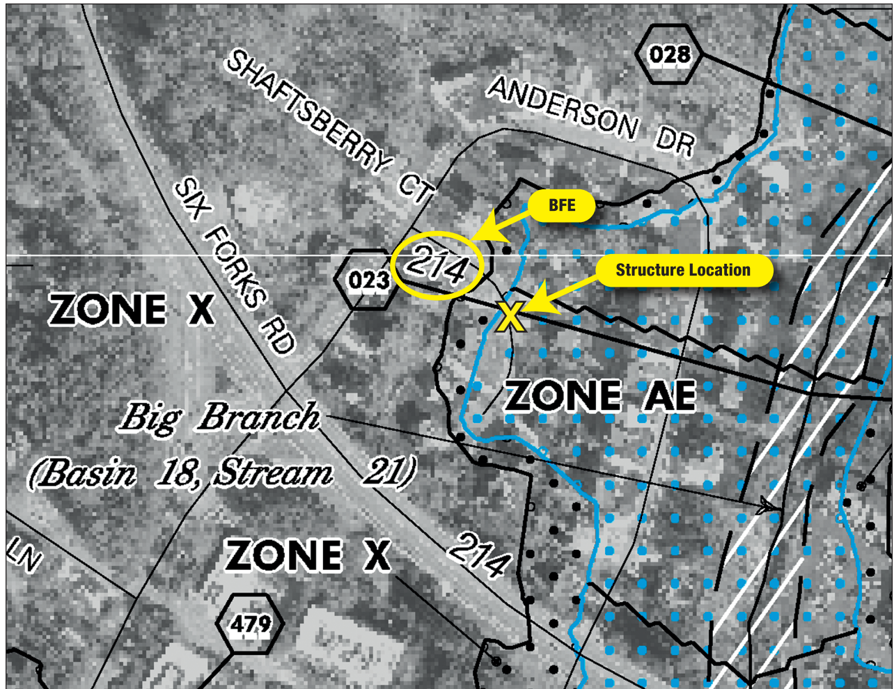
Figure 2-3. Building and stream location on a FIRM
