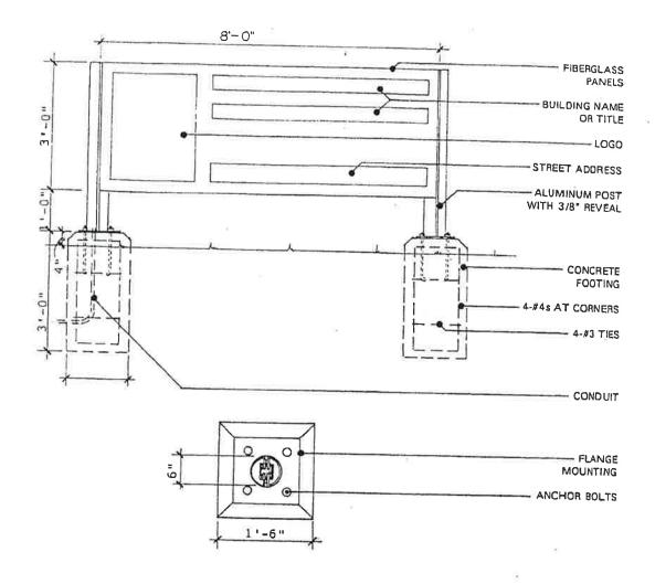
DOUBLE SIDED, REINFORCED FIBERGLASS SIGN WITH ALUMINUM POST.
